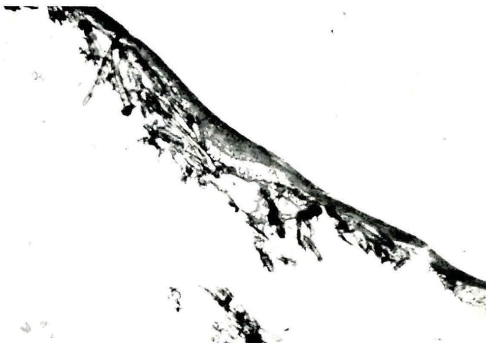
Figure 6. Microscopic photograph of fabric lining the body of the prosthetic pump showing a smooth internal lining with fibrin enmeshed in the fibers of Dacron.
