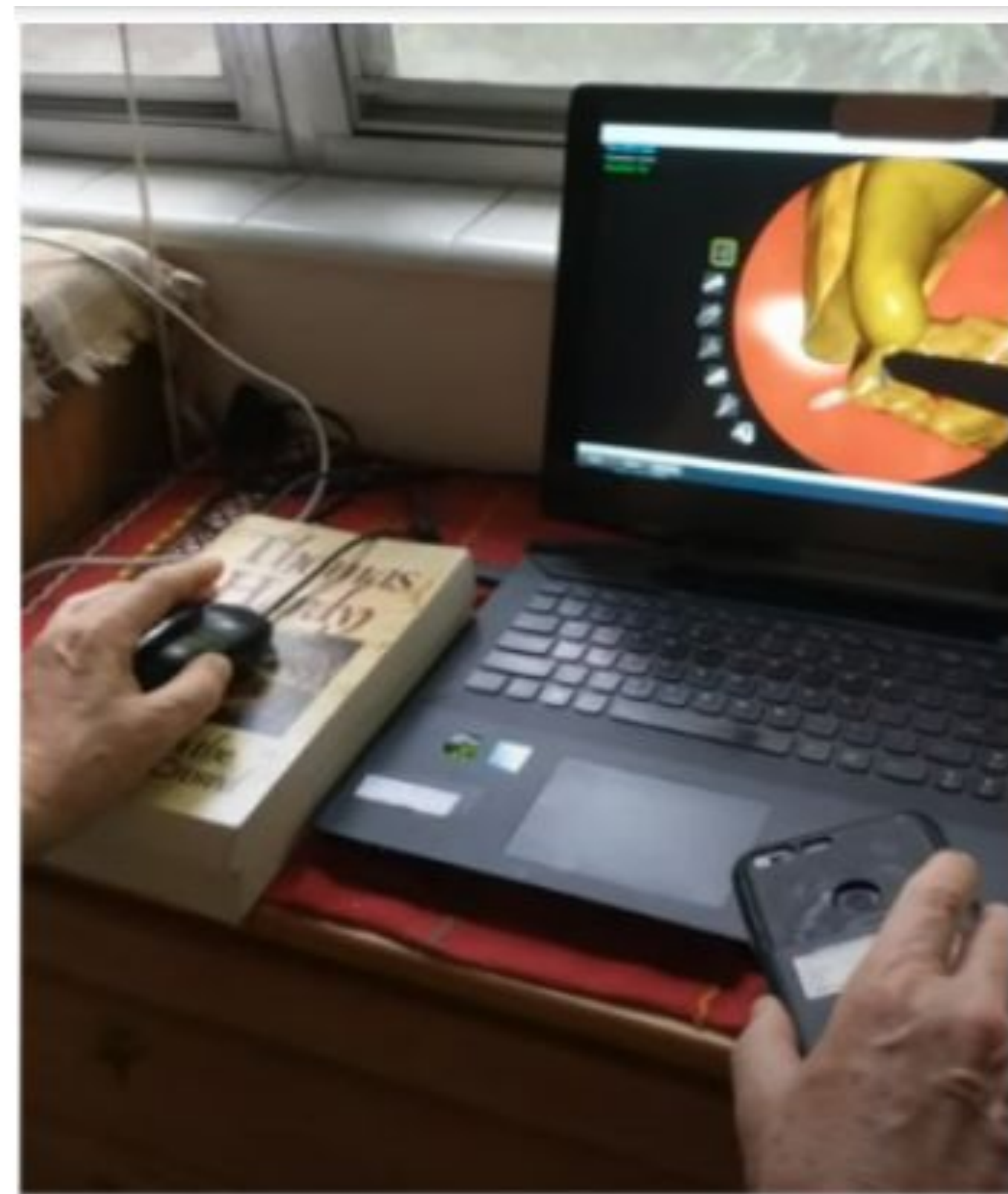
TIPSlite phone-based 4-dof haptic interface (mouse for weak hand) © J.Peters.
