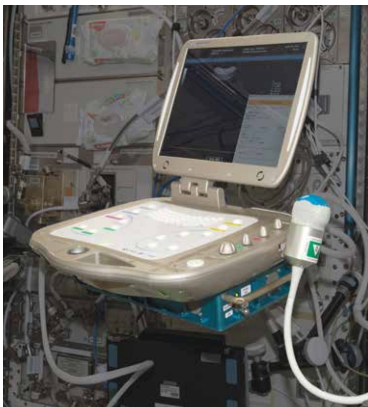
This handheld POCUS machine enables real-time cardiovascular monitoring on the International Space Station. (Credit: NASA)
