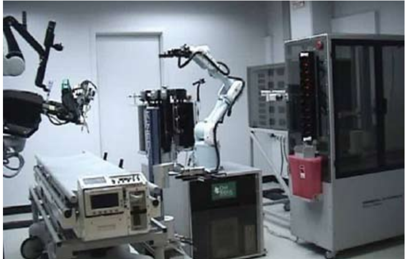
The “operating room without people” project from the military’s Trauma Pod program. To the left are DaVinci robot arms, in the center the “scrub nurse,” in the rear is the tool changer, and to the right is the supply-dispensing “circulating nurse.” (Courtesy of Pablo Garcia, SRI International, Menlo Park, CA, 2006.)
